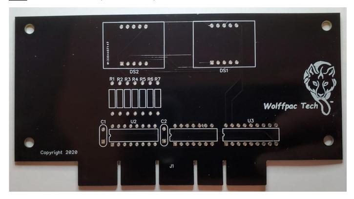
Insert U1 (74HCT32 or 74ACT32) into the board from the top side (the side with the lettering) so that one pin goes through each hole at the location labeled 'U1'. (Note: the marking 'U1' may be hard to read.) Each chip is marked with a 'U'-shaped notch on one of the short ends:
