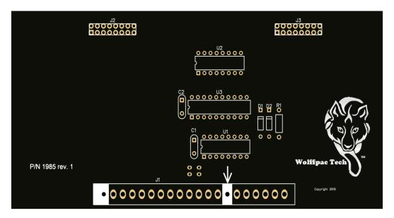
Insert U1 (CD4543) into the board from the top side (the side with the lettering) so that one pin goes through each hole at the location labeled 'U1'. Each chip is marked with a 'U'-shaped notch on one of the short ends:
