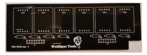
Step 2: Locate resistors R10-R16.
