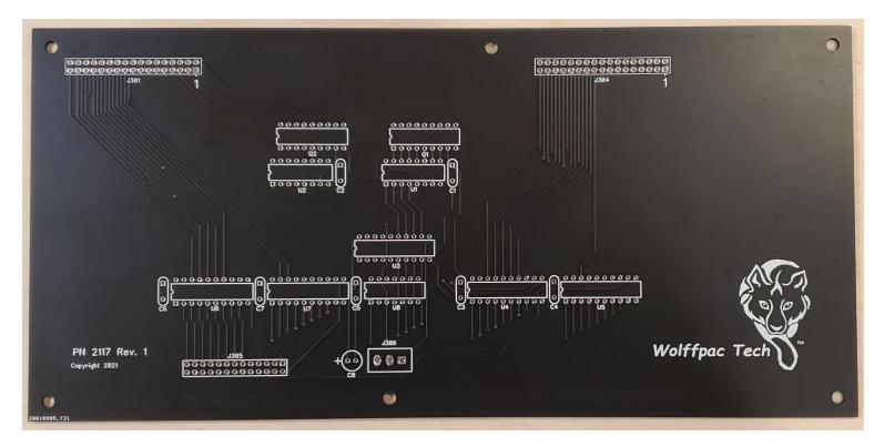
Insert U8 (74ACT32) into the board from the top side (the side with the lettering) so that one pin goes through each hole at the location labeled 'U8'. Each chip is marked with a 'U'-shaped notch (or dot) on one of the short ends:
