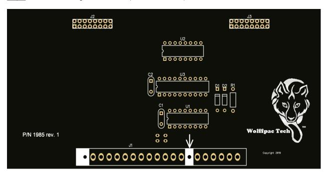
Insert U1 (CD4543) into the board from the top side (the side with the lettering) so that one pin goes through each hole at the location labeled 'U1'. Each chip is marked with a 'U'-shaped notch on one of the short ends:
