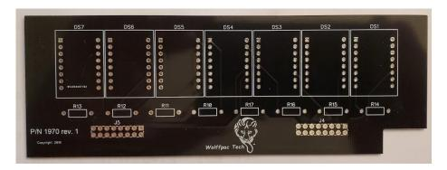
Step 2: Locate resistors R10-R17.
