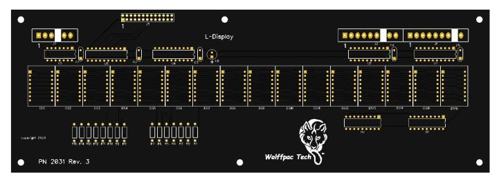
Insert U3 (74ACT08) into the board from the top side (the side with the lettering) so that one pin goes through each hole at the location labeled 'U4'. Each chip is marked with a 'U'-shaped notch on one of the short ends:
