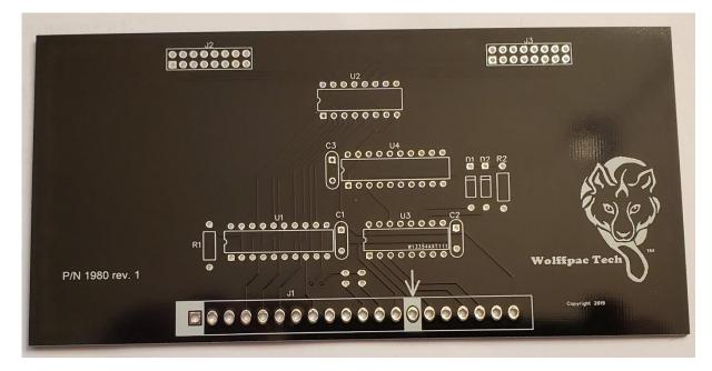
Step 1: Start with the larger PC Board 'A' (marked P/N 1980):
