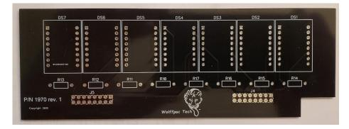
Step 2: Locate resistors R10-R17.
